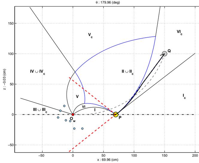
Figure 5.6: Optimal path from points  $Q$  in Region  $VI_c$  ( $S^+T_P^{L+}$  path) ( $Q = [180.27, 33.7^\circ, 12.6^\circ]^T$  and  $P = [70, 0^\circ, 0^\circ]^T$ ) (solid line the real robot trajectory, dashed line the ideal one. Notice that when vehicle is near to spiral  $T_P^L$ , due mainly to localization problem caused by gaussian noise, the vehicle trajectory deviates slightly from ideal one).
