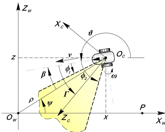
Figure 1.6: Nonholonomic vehicle equipped with a sensor modelled as a planar cone (shaded in figure) which may not include robot's forward direction.  $Z_c$  axis, i.e., axis of symmetry for the sensor, forms an angle  $\Gamma$  with vehicle heading.
