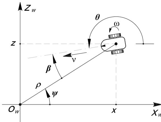
Figure 1.1: Mobile robot and system coordinates  $\langle W \rangle$ .
