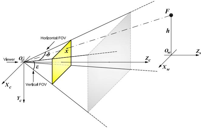
Figure 1.3: Sensor model: four-sided right rectangular pyramid.
