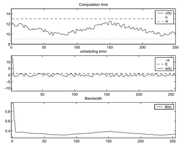
**Figure 3:** First row: computation times  $c(k)$ . Second row: scheduling error evolution. Third row: allocated CPU Bandwidth  $B(k)$
