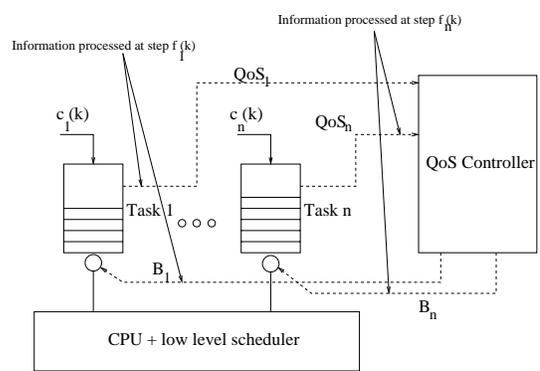
Figure 1: Feedback control scheme for QoS management.
