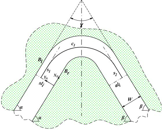
Fig. 4. Sub-optimal path on a turn sector.
