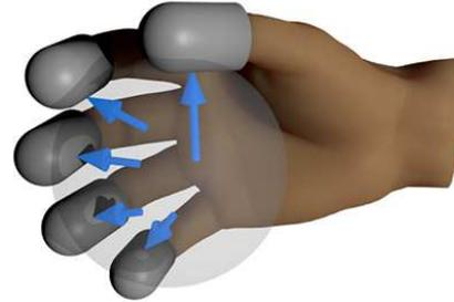
Fig. 1. Concept of the *ThimbleSense* digit-wearable tactile sensor.
