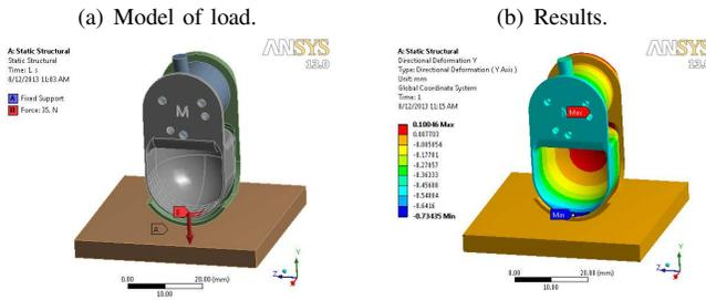
Fig. 4. FEM analysis: load on the inner shell.
