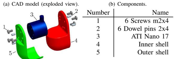
Fig. 6. Shell based wearable device: final design.
