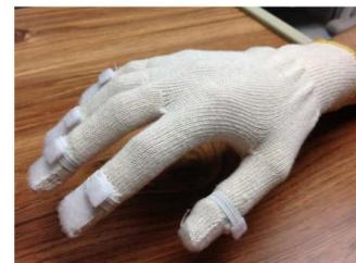
Fig. 7. Glove used to keep thimbles on fingertips.
