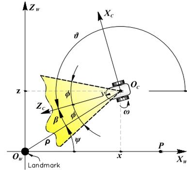
(a) Cartesian and polar coordinates of the robot and H-FOV constraints.
