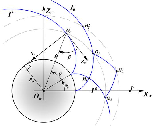
Fig. 3. Extremal arcs for the V-FOV: the involutes of a circle of radius  $R_b$ .  $I_0$  is the involute with  $\psi_b = 0$ . Path  $\mathcal{C}_1 = I^{L+} * I^{R-}$  and path  $\mathcal{C}_2 = I^{R-} * I^{L+}$  both between  $Q_1$  and  $Q_2$ .
