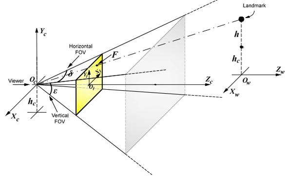
Fig. 2. Sensor model: four-sided right rectangular pyramid with  $\epsilon = 2\hat{\phi}$  and  $\delta = 2\phi$ , where  $\hat{\phi}$  is half of the V-FOV angular aperture, whereas  $\phi$  is half of the H-FOV angular aperture.
