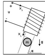
$$\begin{aligned} \dot{x} &= \begin{bmatrix} x_2 \\ \sin(\alpha)g - \frac{c}{m} \left(\frac{x_3}{x_1}\right)^2 \\ -\frac{R}{L}x_3 + \frac{2c}{L} \frac{x_2 x_3}{x_1^2} + \frac{1}{L}u \end{bmatrix} \\ y &= x_1 \end{aligned}$$
