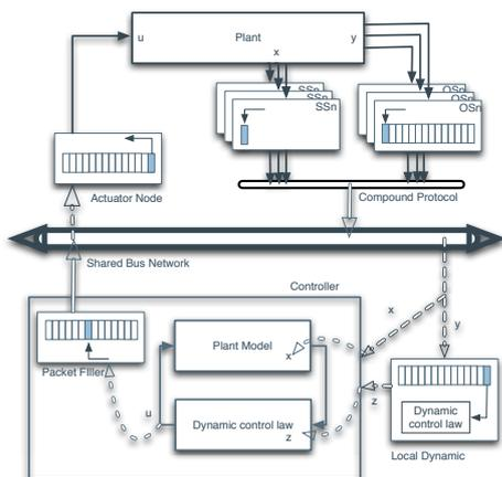
Figure 1: The proposed control architecture
