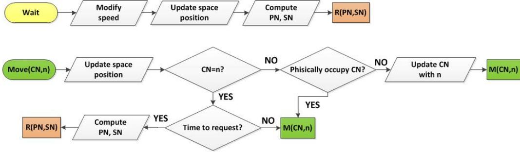
Fig. 3. State flow for agent  $i$  with  $PN_i = n$  and  $SC_i = m$  when waiting for having access to a node or moving toward a new node.
