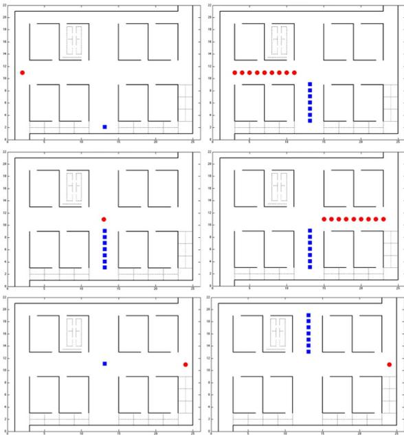
Fig. 6. Two robots in a crossing scenario the lower priority robot waits until the resource is made available. In this scenario for the lower priority robot is not convenient to look for another longer path.
