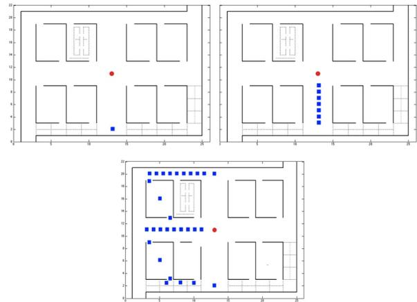
Fig. 8. Evolution of an agent that encounters another agent blocked on a node and after waiting to access that node decides to go toward the goal by replanning.
