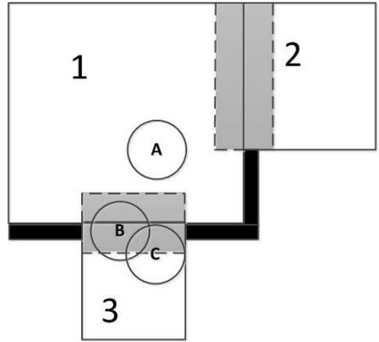
Fig. 4. Consider agent in position  $A$  its current node  $CN$  is node 1, when gained access to 3 and moving toward it, e.g. in position  $B$  the agent is occupying both 1 and 3 in terms of capacity. When an agent reaches position  $C$  it releases node 1.
