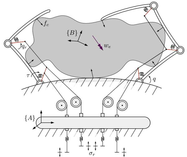
Fig. 1: Compliant grasp by an underactuated robotic hand.
