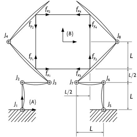
Fig. 4: Compliant grasp of a square by a two fingered spider-like hand.
