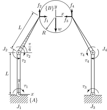
Fig. 2: Compliant grasp of a ball by a two-fingered robotic hand.
