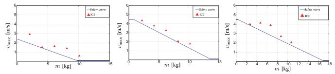
Fig. 17. Conservative safety curves for small sphere (left), large sphere (center), and wedge 45' (right) for robot real-time control. In order to remain well below all observed IC2 injuries, we chose simple shifted regression lines to represent the conservative injury estimates. If the conservative regression line does not intersect with the y-axis before, the minimum and maximum velocity are chosen to be at 0.1 m/s and 4.5 m/s, respectively.
