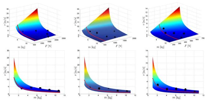
Fig. 29. 3D-plot (upper row) and 2D projection (lower row) of force, mass, and velocity. The black spheres are observed injuries and the red lines an example of speed - mass variation at constant force. The left column shows the results for wedge, while the middle and right one show the forces for the large sphere and the small sphere, respectively.
