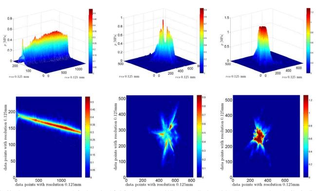
Fig. 30. Impact pressure at 1.5 m/s for the wedge 45° (left), large sphere (middle), and small sphere (right). The upper row shows the 3D visualization and the lower one the impact profile from above. It is easy to observe that only the wedge (line impact) can be measured physically consistent and the pressure profiles of the spherical impactors (2D curvature) are characterized by internal tension caused by the incapability of the foil to bend in 2D.
