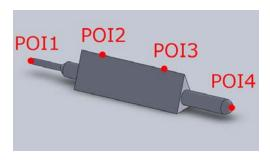
Fig. 21. End-effector composed of impactor primitives and the associated POIs. POI1 is attached to the small sphere, POI2, POI3 to the edge, and POI4 to the large sphere. Please note that the corners of the end-effector have not been drop tested yet. Therefore, we omit their effect on the POI selection, i.e. we assume the corners to be roundish.
