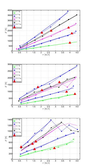
Fig. 28. Impact forces against impact velocity. The upper plot shows the results for the wedge, while the middle and lower one show the forces for the large and small sphere, respectively.
