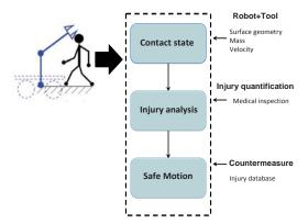
Fig. 4. Proposed methodology. Based on the mechanical *input parameters* mass, velocity, and surface geometry, a medical evaluation leads to the quantification of injury. The relation between them can then be used for a control strategy that ensures safe motion behavior.
