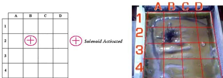
**Fig. 7.12.** Psychophysical experimental setup: top-view of the HBB-I workspace with alphanumeric coordinates of 16 quantized points (left) and real activation of one point having coordinate  $B2$  (right).
