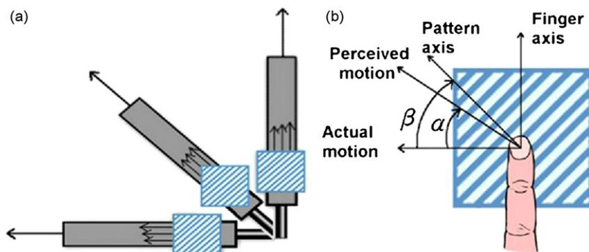
Fig. 1. The apparatus for the tactile barber-pole experiment. (a) Textured pad mounted on a motorized slide moving towards three different directions. (b) The angle  $\alpha$  is between the perceived and actual directions of motion (on the vertical axis) while the angle  $\beta$  is between the actual direction of motion and the axis of the pattern on the pad for three different motion directions.
