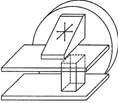
Figure 2: A parallel-jaw gripper can manipulate polyhedral parts
