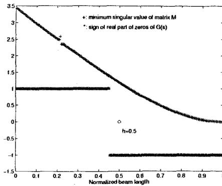
Figure 2: Cost function and constraints for the optimal design problem, computed with a 3-modes model. +: minimum singular value of  $M$ . \*: sign of the maximum real part of the zeros of  $G(s)$ . o: suggested sensor placement accordingly to the defined criterion
