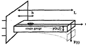
Figure 1: The physical system considered. A beam of length  $L$ , fixed at one end and free at the other end, is subject to a time-varying force  $F(t)$  applied at the free end which causes transverse vibrations  $y(x, t)$ . A strain gauge, placed at a position  $h$  along the beam, is used to estimate the applied force.
