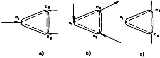
Figure 2: Active and preload internal forces for the grasp of fig.1
