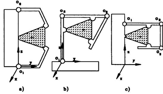
Figure 3: Three different manipulators grasping the same object.
