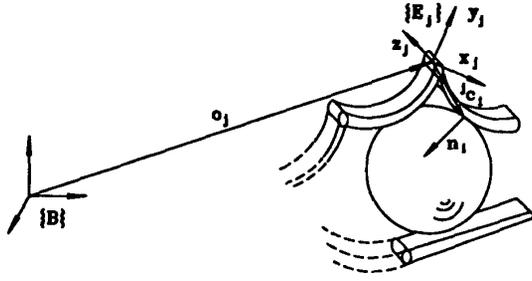
Figure 1: Local and base reference frames in cooperating manipulation.
