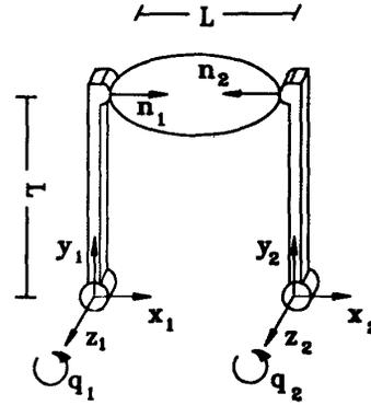
Figure 2: Two one-link manipulators holding an object.
