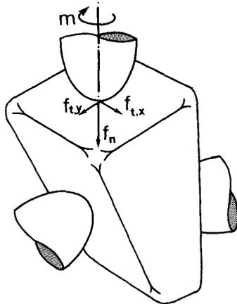
FIG.5: Resultant friction force and torque in a 3D grasp.
