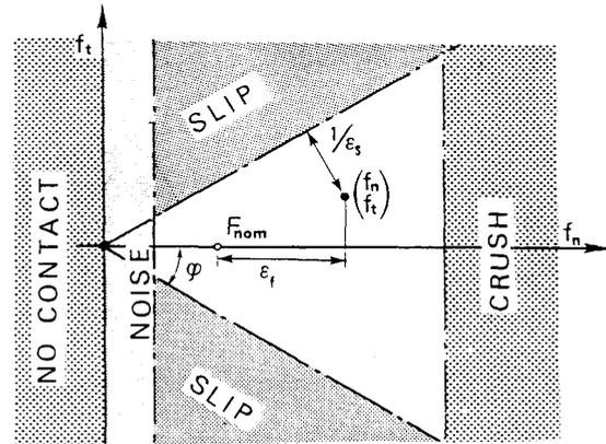
FIG.2: Unacceptable contact conditions in  $f_n$ - $f_t$  plane
