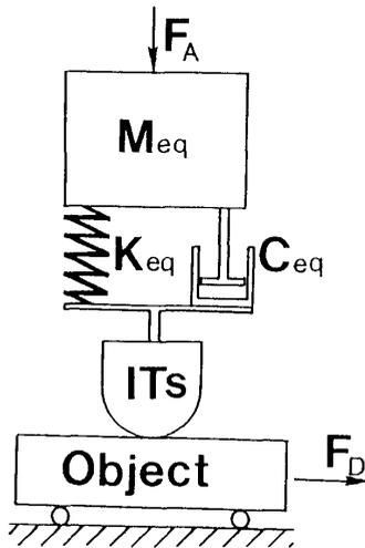
FIG.7: Simulation model for the active finger - object system.
