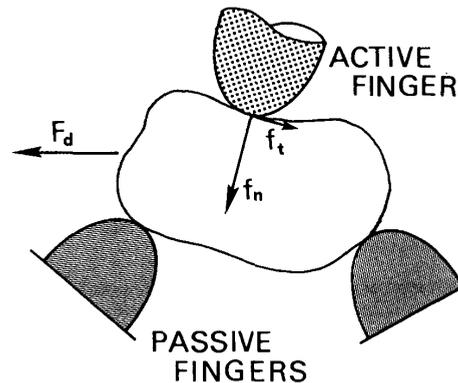
FIG.1: Planar grasp with one active finger.
